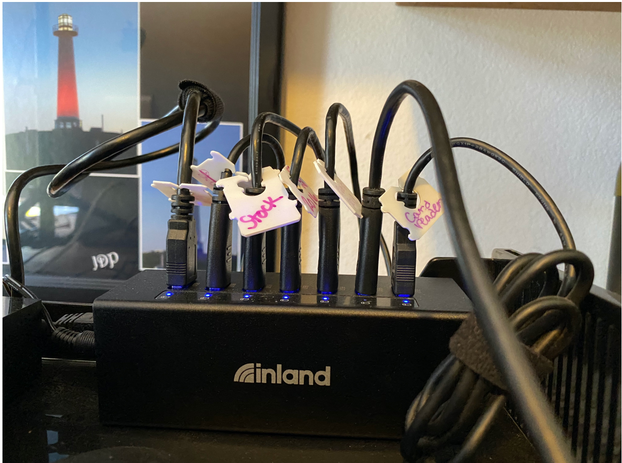
Figure 1 Seven-port hub with bread ties to identify connected drive
